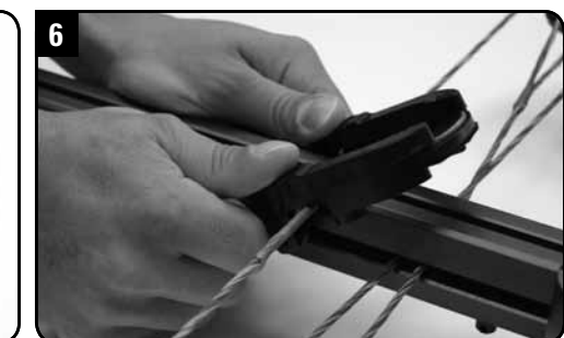
Connect the string slots to the bowstring and lower the guidepost into the barrel's flight groove.
