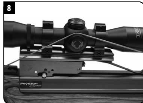
Don't allow the draw cord to get hung-up on any part of the crossbow, scope or accessories.
