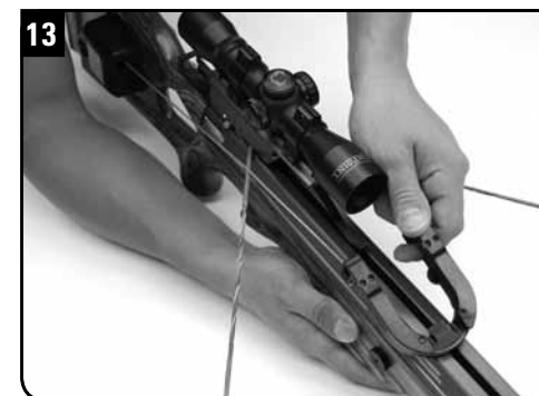
Once you relieve the string tension on your cocked crossbow, remove the crank so you can slide the claw forward.
