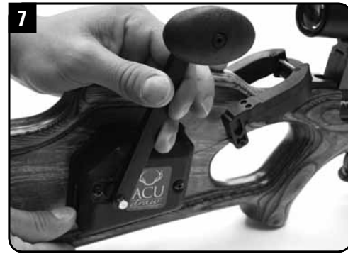
Relieve the tension on the ACUdraw™ unit before lifting the claw out of its storage position (approximately ¼-inch to ½-inch).
