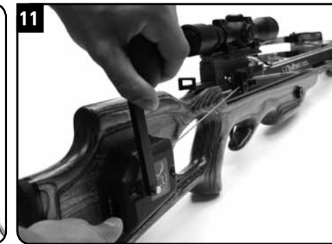
To avoid damaging your ACUdraw™ once your bow is cocked, apply a small amount of additional clockwise pressure to the crank (approximately ¼-inch to ½-inch), disengaging the safety pawl and unwind the mechanism 2 ½ to 3 turns to relieve the string tension.
